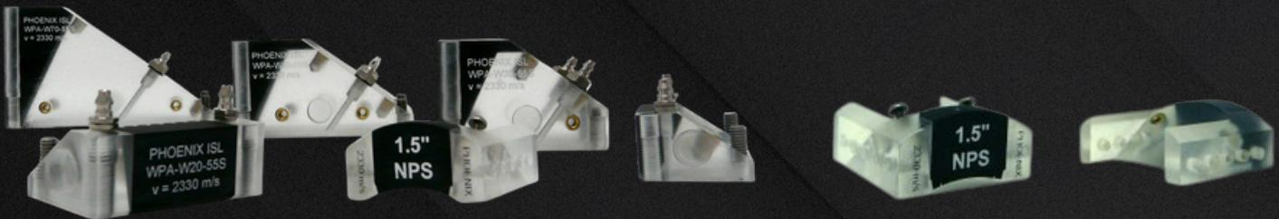
Wedges are used in both shear wave and longitudinal wave applications, including straight beam linear scans. These wedges perform basically the same function in phased array systems as in conventional single element flaw detection, coupling sound energy from the transducer to the test piece in such a way that it mode converts and refracts at a desired angle in accordance with Snell's Law.
